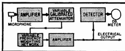
Fig. 23-7. Basic block diagram of a sound-level meter.
