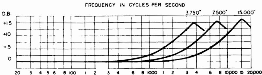
Fig. 12-38. Frequency vs. amplitude characteristics of the PT63-A.
