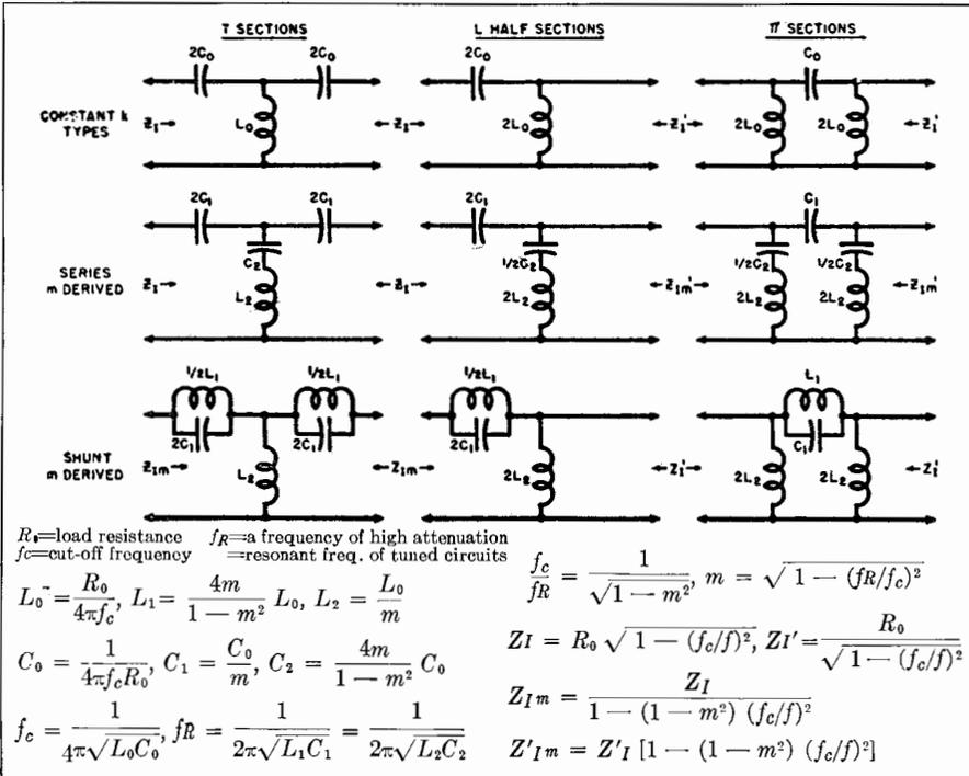
Table 6. Information for the design of high-pass filter sections.
