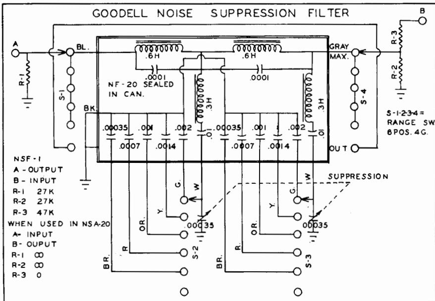
Fig. 17-26. Schematic of the NSF-2 noise suppression filter.
