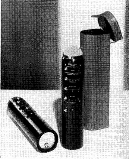
Fig. 28-45. The Scott 410-A Sound Level Meter.
