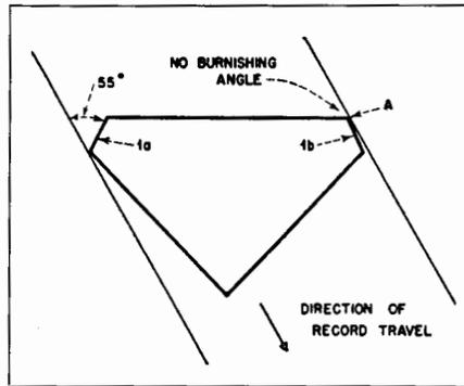
Fig. 7-12A. Same stylus cross-section in groove whose slope is  $30^\circ$ . Burnishing facet 1a forms angle of  $55^\circ$  with adjacent wall. Facet 1b cannot burnish with groove slope in excess of its basic angle. In fact, the edge formed by the meeting of cutting face and burnishing facet (A) will tear the adjacent groove wall. (Courtesy, F. L. Capps)
