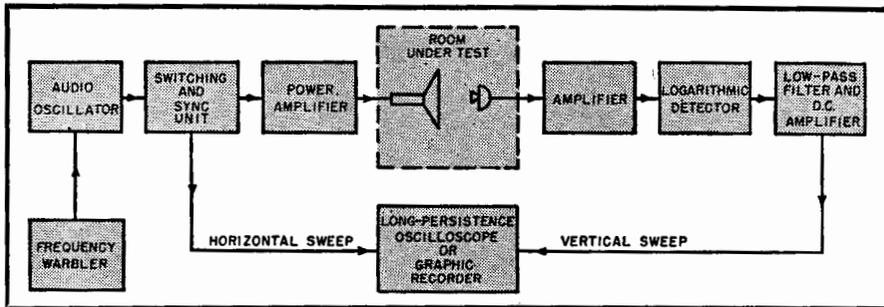
Fig. 23-4A. Measurement setup for determining reverberation time.
