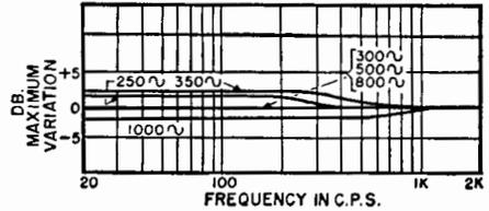
Fig. 20-12. Max. error in l.f. response resulting from use of 300-, 500-, and 800-cycle equalization for 250-1000 turnover points.
