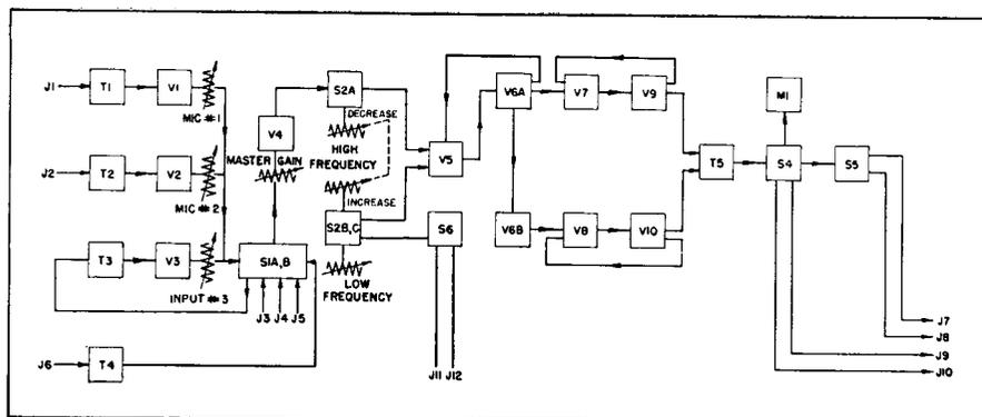
Fig. 26-34. Block diagram of the 90-B recording console.
