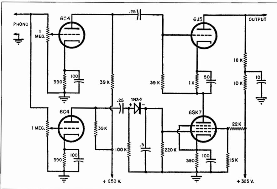
Fig. 19-44. Typical voltage amplifier circuit, incorporating the expander.
