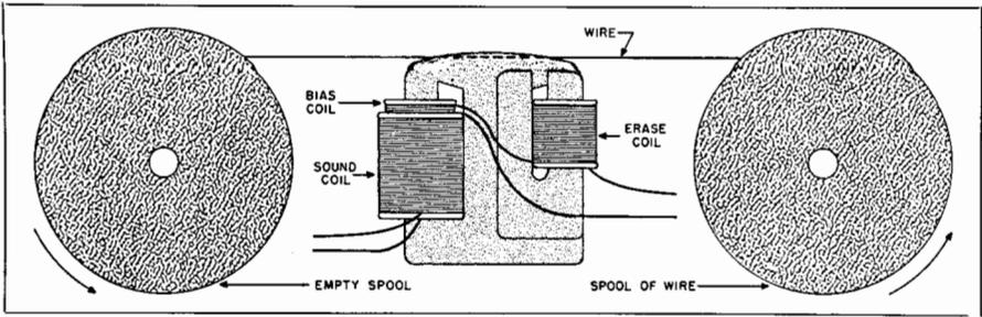
Fig. 3-20. Combined record-playback head assembly for wire.
