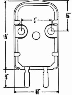
Fig. 9-36. Cut-away drawing shows the novel construction of the Model 12D cartridge.
