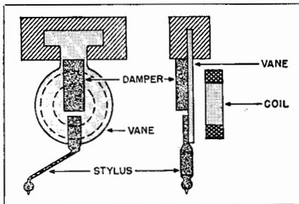
Fig. 9-12. Moving vane structure of Zenith "Cobra" pickup.
