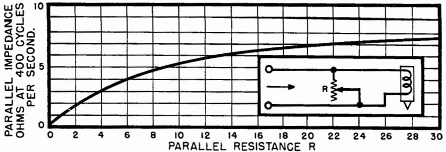
Fig. 4-17. Chart used to determine parallel 400 cycle impedance.
