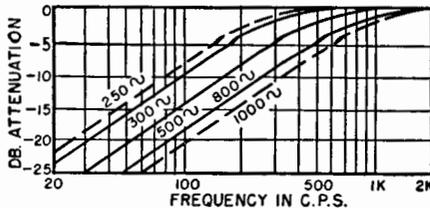
Fig. 20-10. Typical low frequency attenuation for various turnover frequencies as used in recording different phonograph discs.
