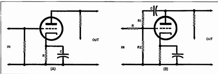
Fig. 17-5. (A) This circuit will boost the higher frequencies when condenser  $C$  is of too low a value to provide an adequate bypass for the cathode resistor at the reference and lower frequencies. (B) By choosing component values, this circuit can provide inverse feedback on the highs.
