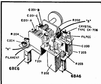
Fig. 24-4. Details show compactness of AM tuner sub-chassis.
