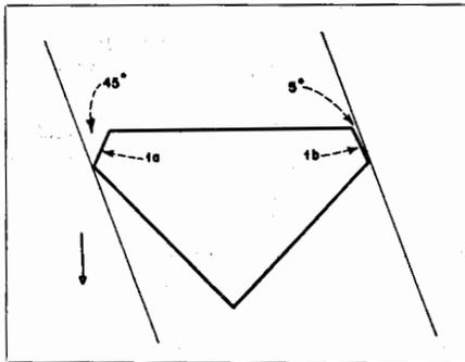
Fig. 7-11. Cross-section of same stylus in groove with  $20^\circ$  slope. Change in angular relationship between burnishing facets and groove is shown. Facet 1a forms angle of  $45^\circ$  with adjacent groove wall. Facet 1b on opposite side of stylus forms angle of  $5^\circ$  with its adjacent wall. In this and subsequent illustrations groove slopes in the opposite direction will merely reverse the effects described. (Courtesy, F. L. Capps)
