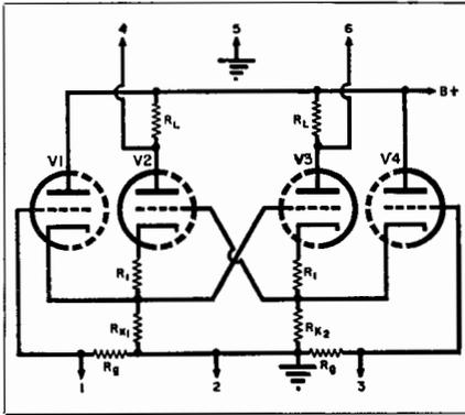
Fig. 19-16. Basic schematic of the cross coupled input circuit.
