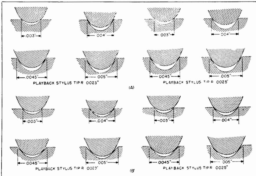
Fig. 7-8. Theoretical seating of stylus in grooves of various widths. (A) Grooves cut with 70° stylus, (B) grooves cut with 90° stylus. (Tip radius .0017") (Courtesy, RCA)
