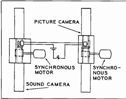
Fig. 3-16. Synchronization of sound and picture cameras.
