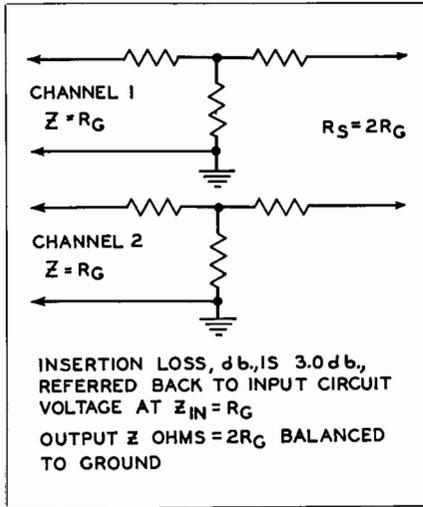
Fig. 18-7. The Two Channel series mixer.
