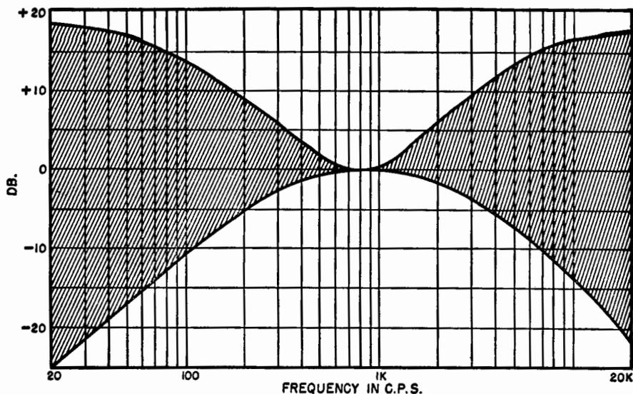
Fig. 21-10. Over-all range of the treble and bass controls of the C-5 preamp-equalizer.
