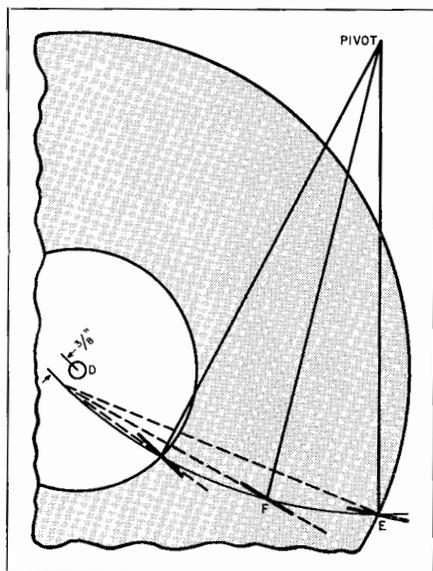
Fig. 10-3. Reproducing needle swings in arc below hub line.
