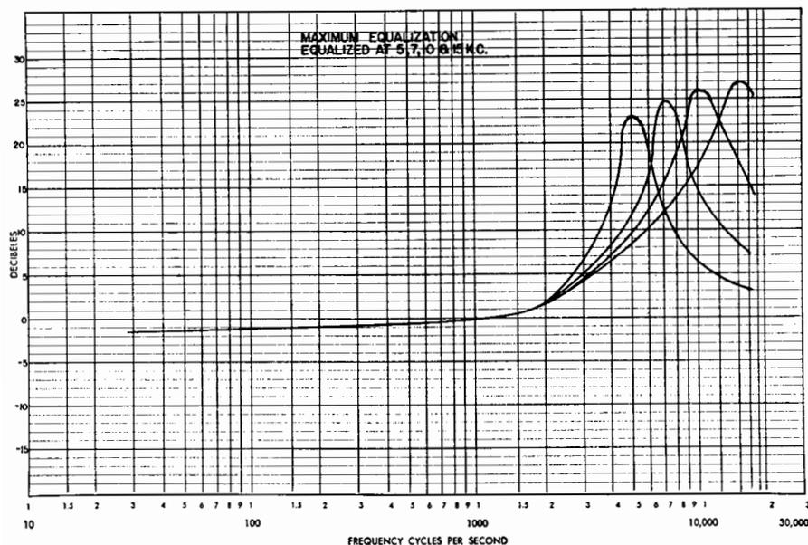
Fig. 17-34. Equalized characteristics of the high-frequency equalizer.
