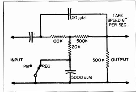
Fig. 12-9. Equalizer circuit for magnetic tape recording.
