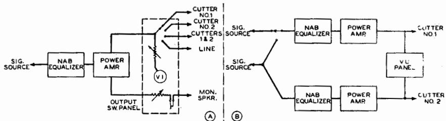
Fig. 26-25. Alternate arrangements for feeding two recorder channels.
