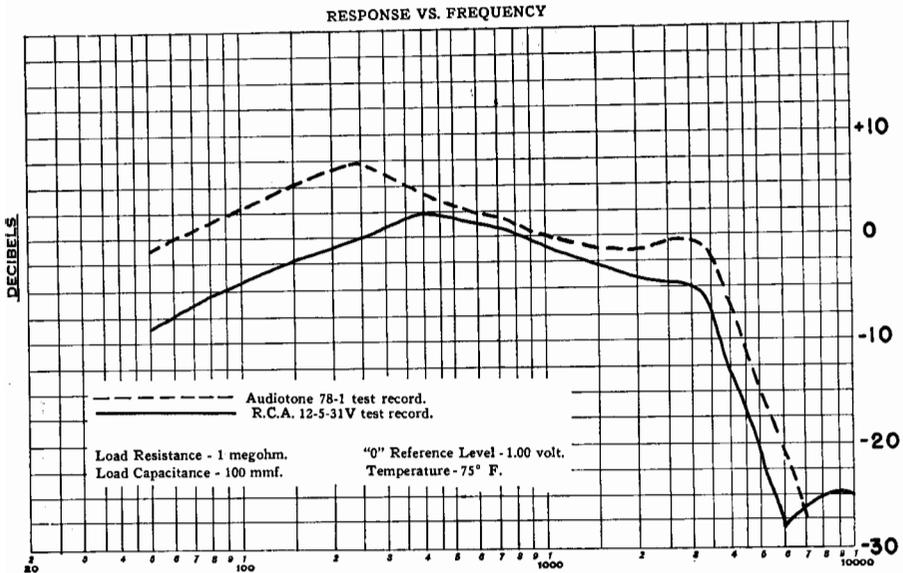
Fig. 9-33. Response curve of the ACD-1J cartridge.
