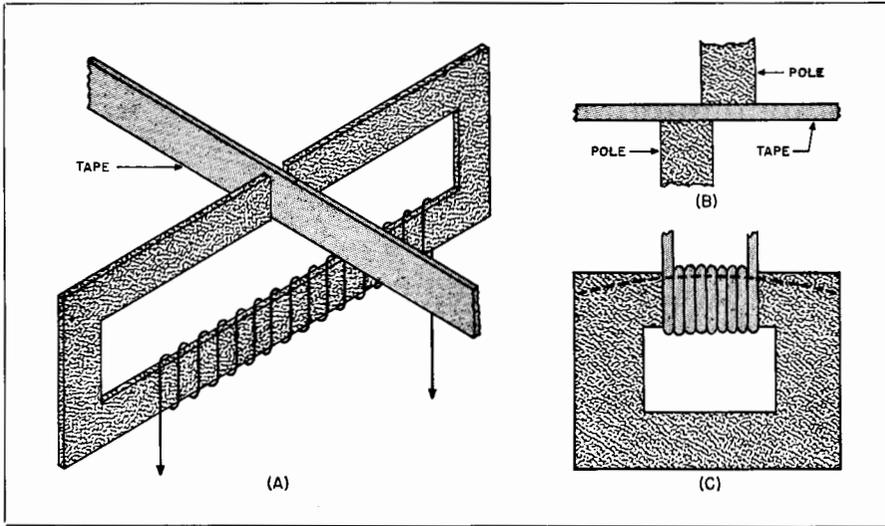
Fig. 11-11. (A) Record-reproduce head for transverse recording on tape. (B) Offset thick pole pieces used to improve characteristics of head shown in (A). (C) The closed wire head used in some types of magnetic recorders.
