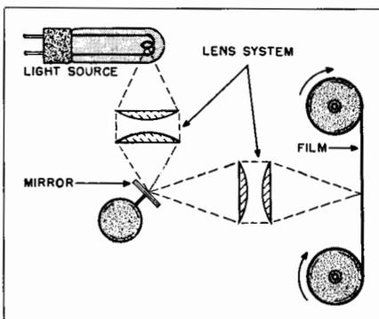
Fig. 3-7. The essential elements used for variable area optical recording.
