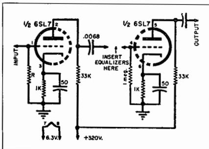
Fig. 20-1. Circuit diagram of preamplifier.
