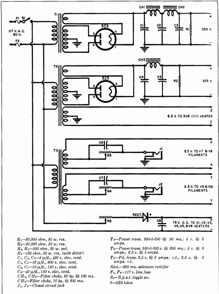
Fig. 19-37. Schematic diagram of the power supplies. Outputs are fed to amplifier through heavy cable. Plate current may be measured at jacks, *J*<sub>1</sub> and *J*<sub>2</sub>.
