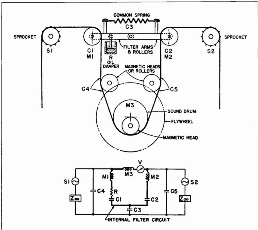
Fig. 13-2. Film path schematic and equivalent electrical circuit.
