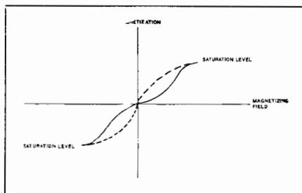
Fig. 11-15. Characteristic curve of a magnetic medium.
