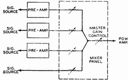
Fig. 26-28. Set up for multiple channel mixing.
