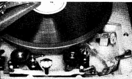
Fig. 5-17. A brake shoe is applied to the turntable rim and rubber idlers are removed from contact in the "off" position.
