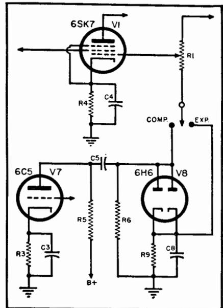
Fig. 19-33. Necessary change in expander circuit in order to obtain Volume Compression.
