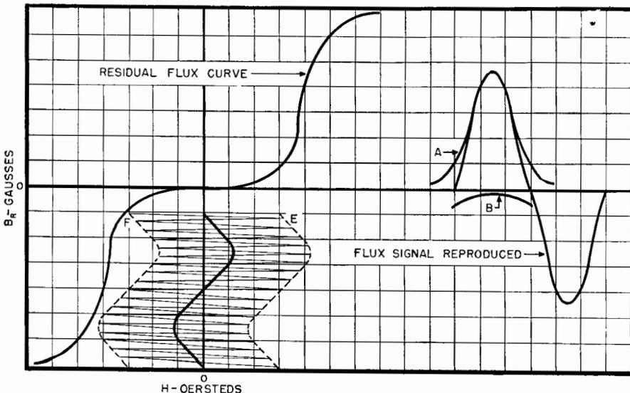
Fig. 11-9. Ultrasonic biasing effect. Combined audio and ultrasonic magnetizing field is applied to residual flux density curve to plot the flux signal that the wire will produce in the gap.
