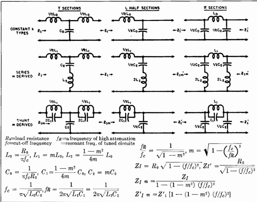
Table 5. Information for the design of low-pass filter sections.
