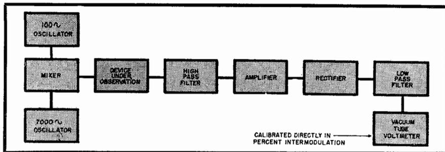
Fig. 28-7. Block diagram of a basic intermodulation meter.
