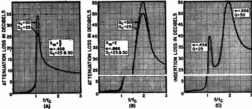
Fig. 16-21. (A) and (B) Attenuation curves of two different networks with different values of  $m$ , for two values of  $Q$ . (C) Attenuation characteristic of a composite filter made up of two of the sections shown in (A) and (B).
