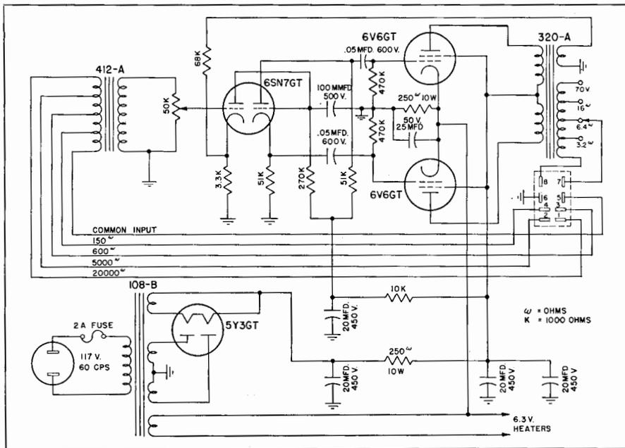
Fig. 25-15. Schematic of Langevin type 130A monitor amplifier.
