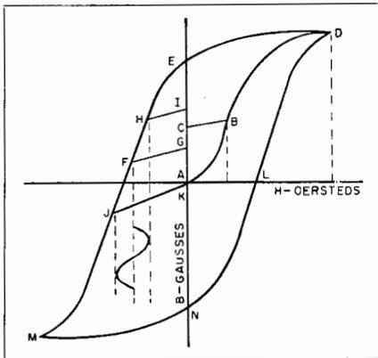
Fig. 11-7. Typical magnetic material magnetization characteristics.
