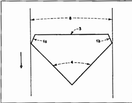
Fig. 7-10. Cross-section of standard lacquer recording stylus in unmodulated groove. Burnishing facets (1a and 1b) form  $25^\circ$  angles with groove walls (8). Arrow shows direction of record travel. Other facets: Cutting face (3) and clearance faces (4). (Courtesy, F. L. Capps)
