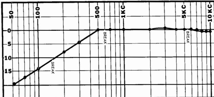
Fig. 28-42B. Frequency response curve of No. 2000S.
