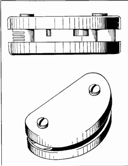
Fig. 12-20. Details of the dual track record-reproduce head.
