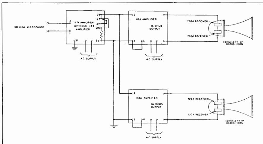
Fig. 22-5. Simple outdoor announcing system, using horn projectors.
