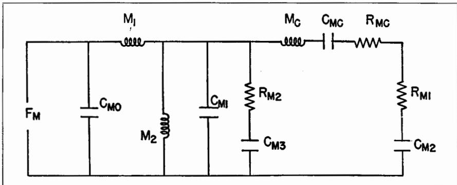
Fig. 9-23. Electrical circuit for a Bimorph phono cartridge.
