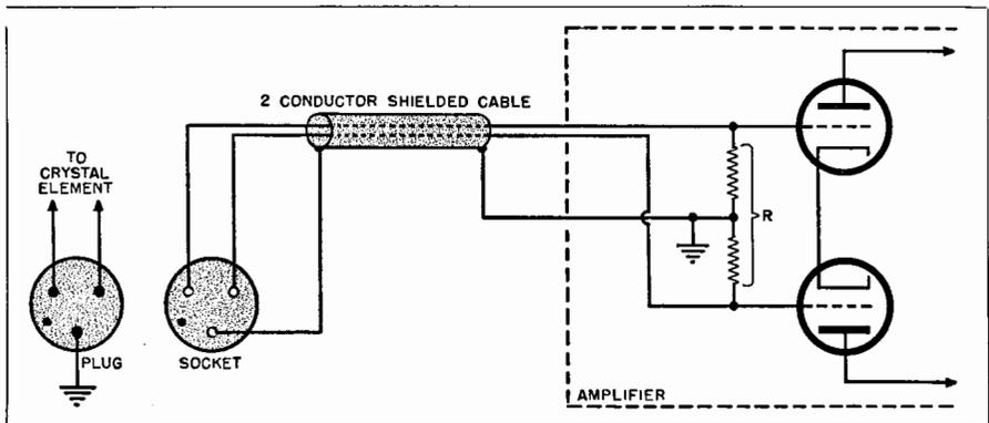
Fig. 14-5. Input connections for sound cell microphones.
