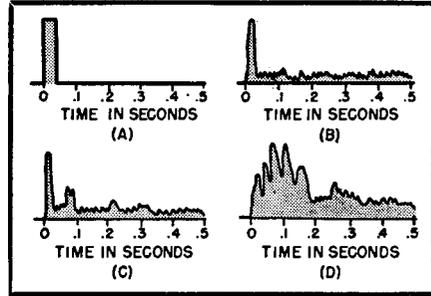
Fig. 23-11. Pulse patterns showing results of transient characteristic measurement on several different theaters.
