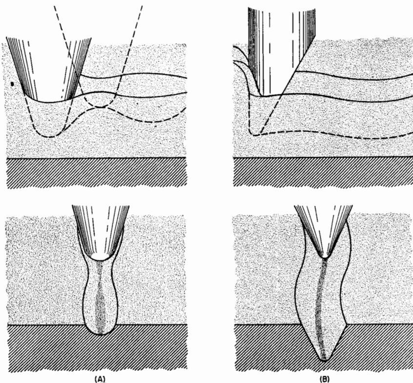
Fig. 3-3B. (A) Embossing action of a dull stylus moving vertically. (B) Engraving action of a cutting stylus that is moving laterally.
