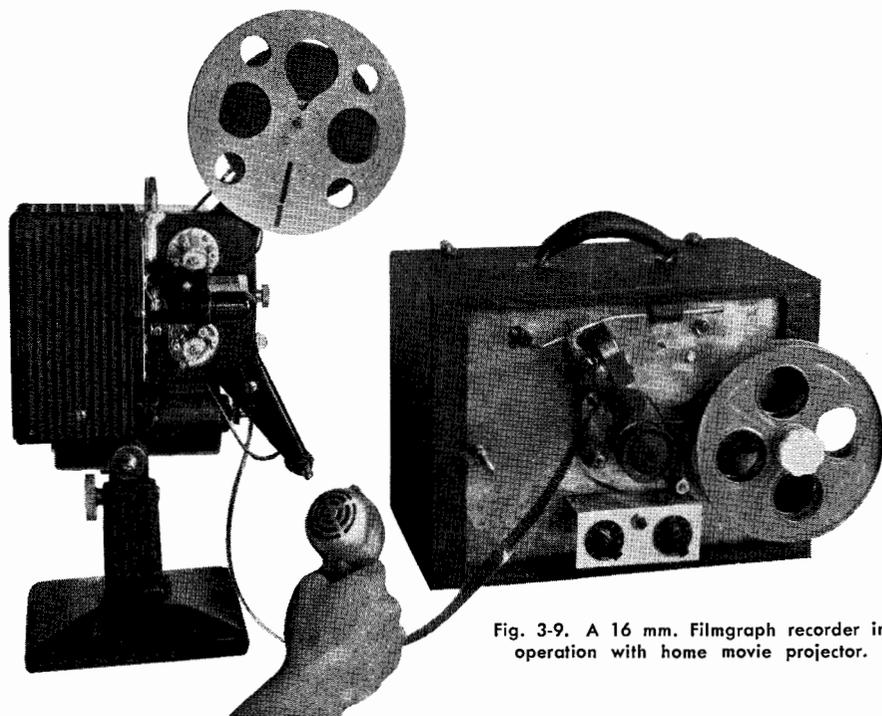
Fig. 3-9. A 16 mm. Filmgraph recorder in operation with home movie projector.
