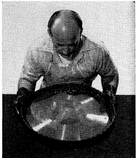
Fig. 27-1. Silverplating the "master" recording.
