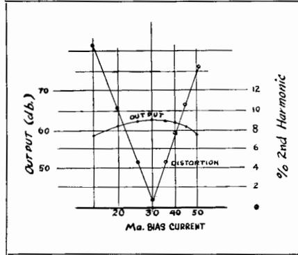
Fig. 11-23. Output and Distortion vs. Bias Current.
