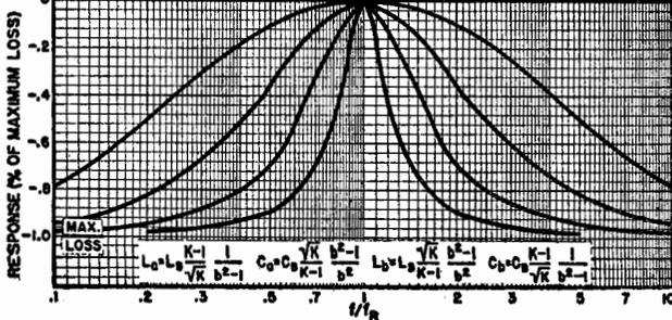
Table 2. Formulas and curves for equalizer design using several different networks for the  $Z_a$  and  $Z_b$  arms.
