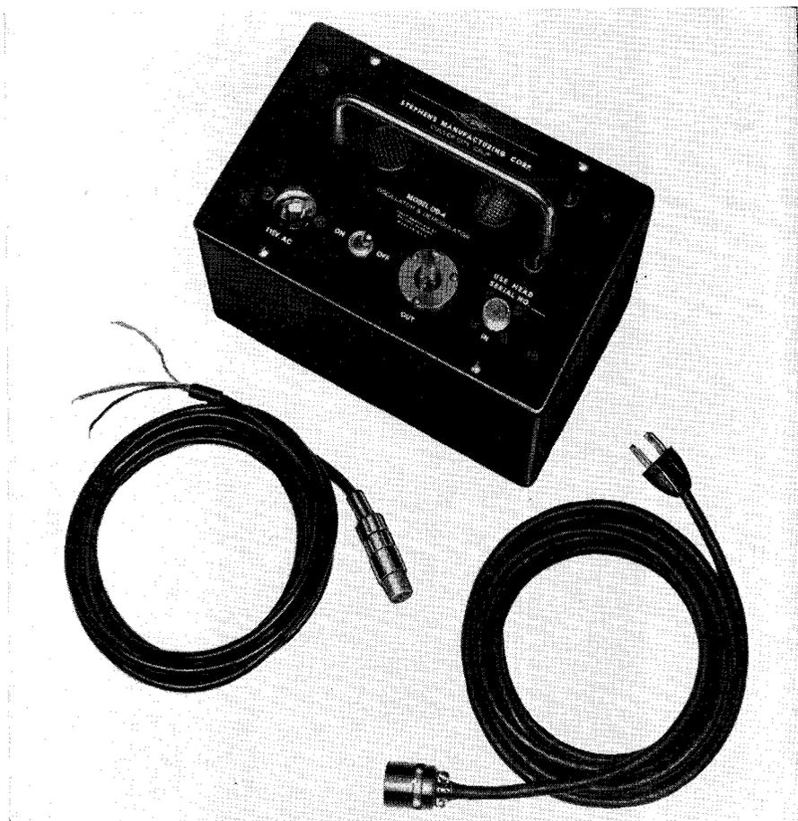
Fig. 14-34. Stephens oscillator-demodulator unit type Model OD-4. (Courtesy Stephens Manufacturing Corp.)
