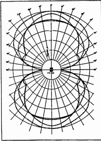
*Directional characteristics of a typical 44-BX Velocity Microphone*
