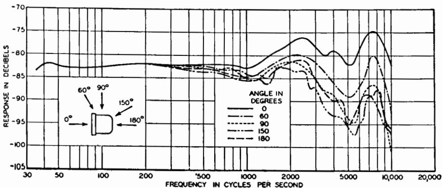
Fig. 14-9. Angular response of moving coil microphone.
