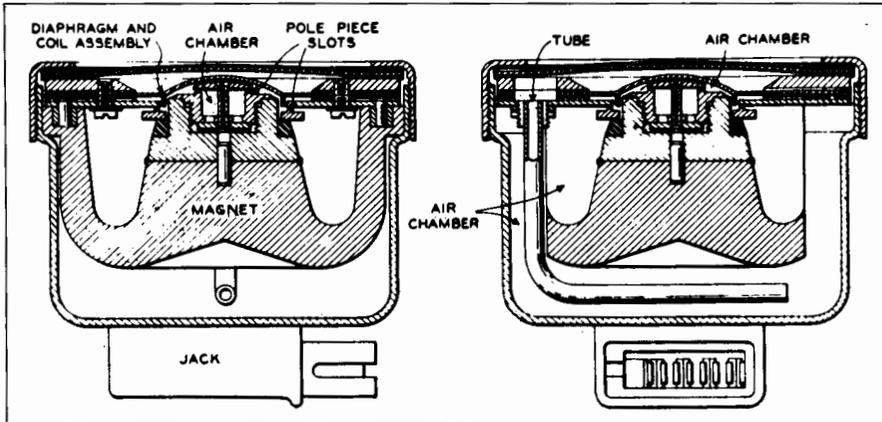
Fig. 14-8. Cross-section view of moving coil microphone.
