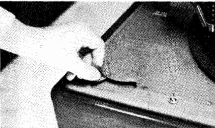
Fig. 5-15. A single "off-on" lever controls both synchronous turntable drive motors.
