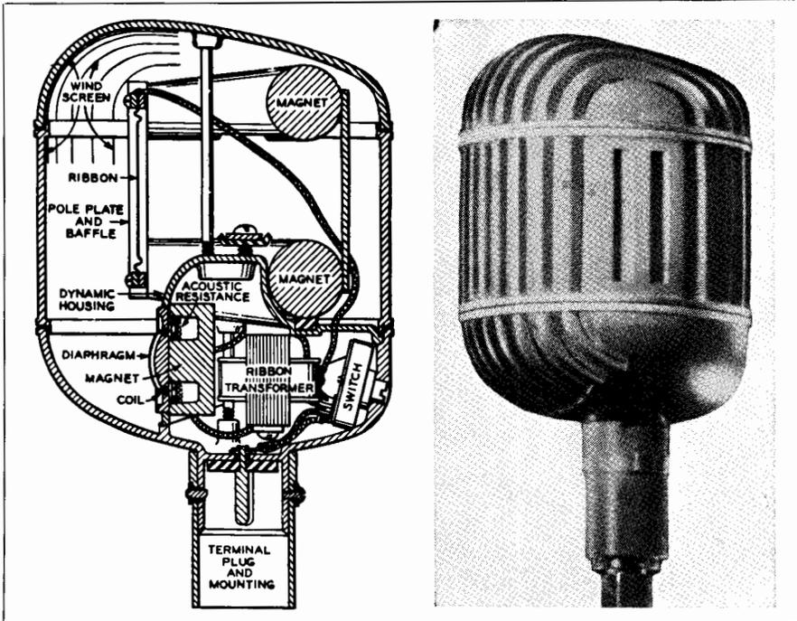
Fig. 14-16. The Western Electric 639-A cardioid directional microphone.
