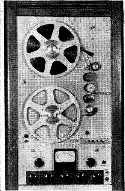
Fig. 12-25. The Presto RC-10/24 Magnetic Tape Transport Mechanism and Amplifier. (Courtesy Presto)
