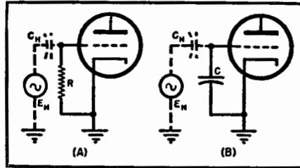
Fig. 28-32. (A) Capacitive hum pickup. (B) Capacitive hum pickup in crystal microphone or phonograph input circuits.
