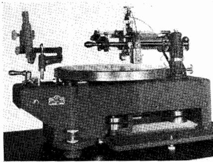
Fig. 5-35. The Presto Model 8D professional disc recorder. (Courtesy, Presto Mfg. Co.)
