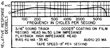
Fig. 12-11. Typical frequency response curve. Low and high frequency ends have been boosted to give flat frequency response.
