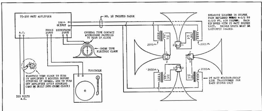
Fig. 22-15. A 75-100 watt church steeple installation. (Courtesy University)
