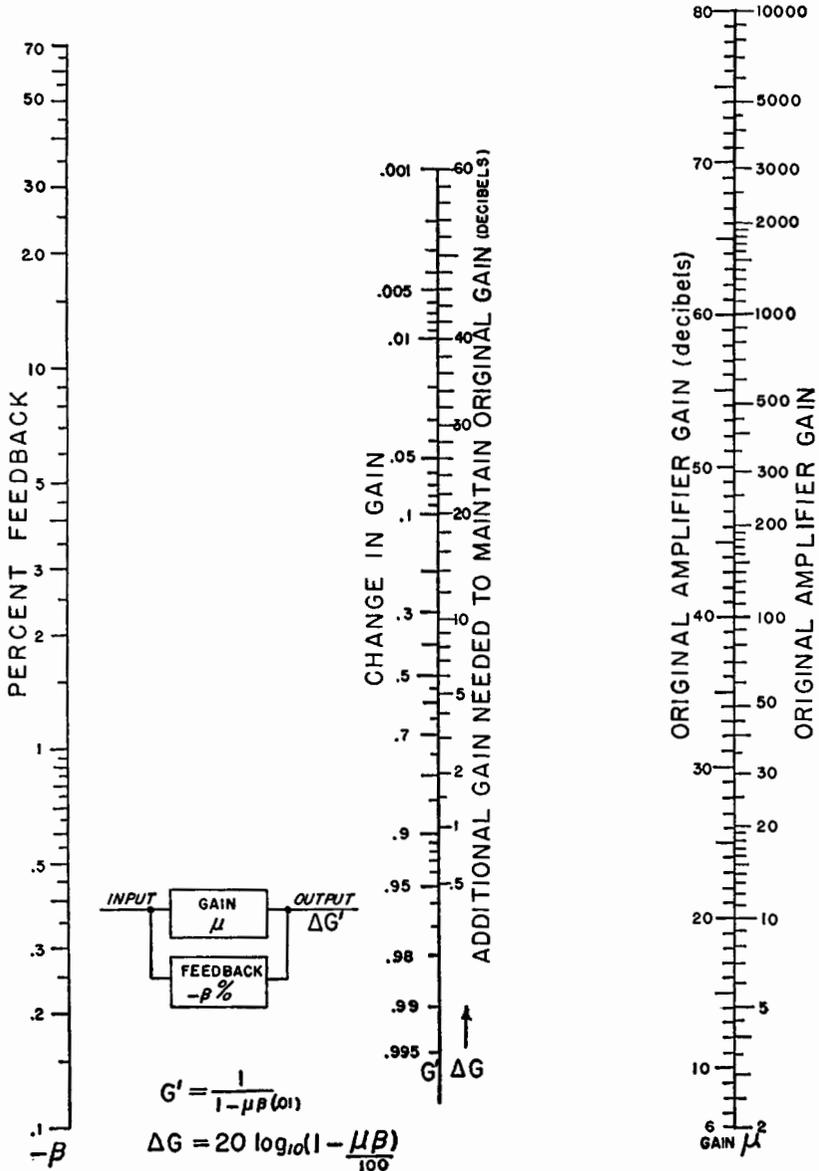
In negative feedback amplifier considerations  $\beta$  (expressed as a percentage) has a negative value. A line across  $\beta$  and  $\mu$  scales will intersect center scale to indicate change in gain resulting. It also indicates amount (in decibels) by which input must be increased to maintain original output. Original amplifications may be expressed as voltage ratio in decibels by using appropriate scale at right.
