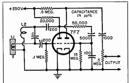
Fig. 9-13. Movement of pickup stylus amplitude-modulates an oscillating detector amplifier. Audio signal is obtained at output.
