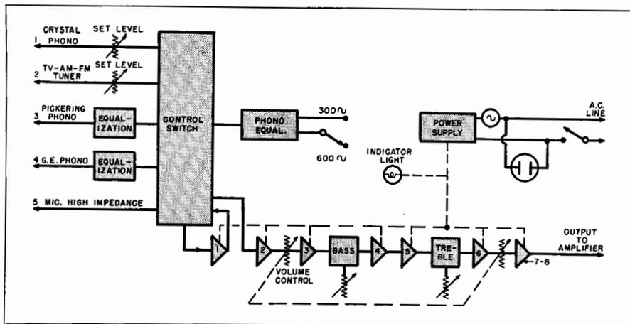
Fig. 26-6. Block diagram of the AE-2 combined preamp-equalizer.
