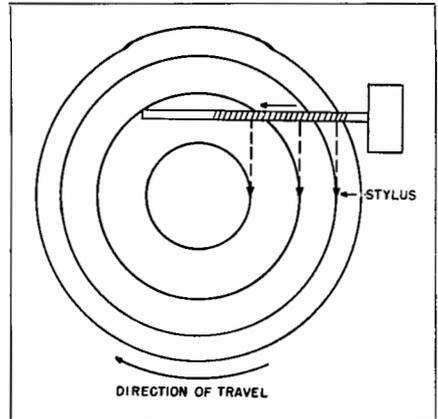
Fig. 5-6. Professional type drive mechanism maintains perfect tangency to the groove.
