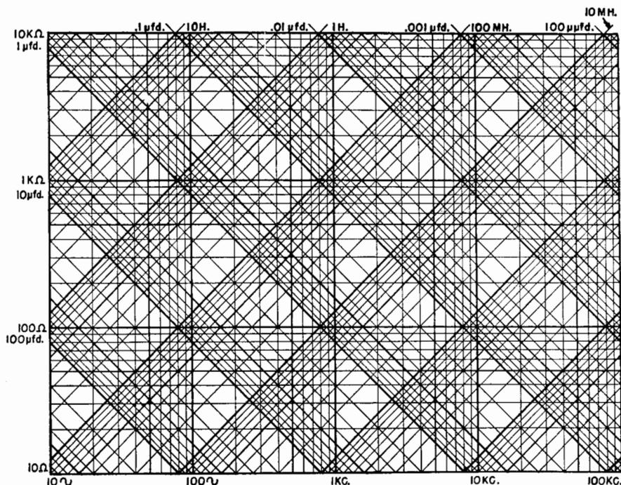
In designing an electrical filter, it is customary to determine the constants of the elements to a fairly high degree of accuracy. However, the damping characteristic of the constant  $K$  type filter is not sharp, so that calculations to an accuracy of better than a few per-cent are seldom required, and effective use can be made of charts to determine inductance and capacitance.
