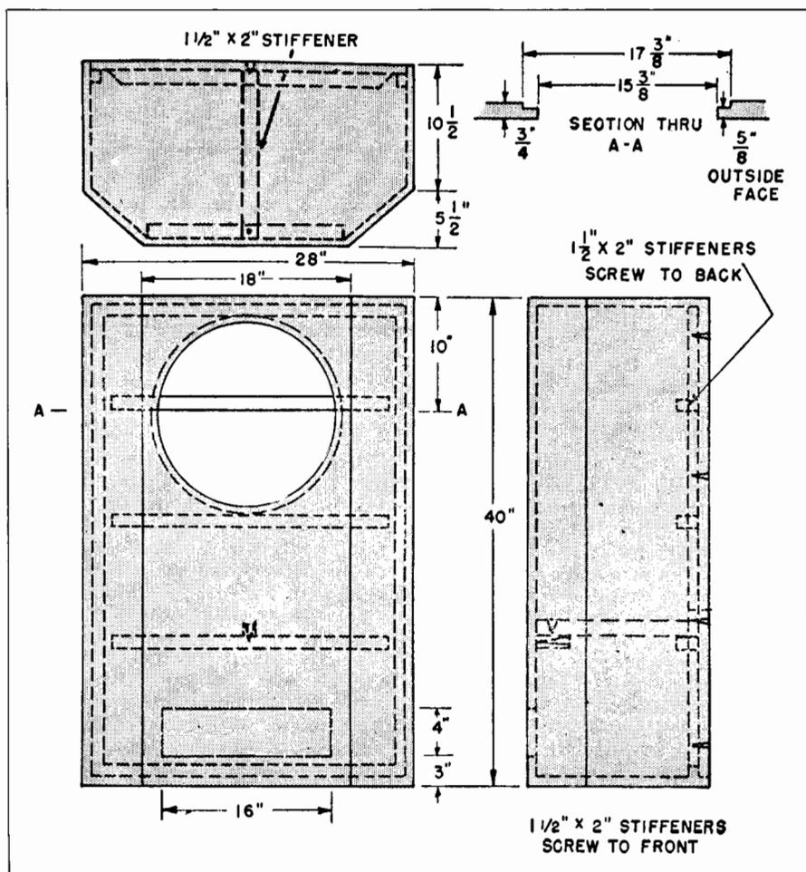
Fig. 15-32. Front, plan and side views of a properly designed loudspeaker housing.
