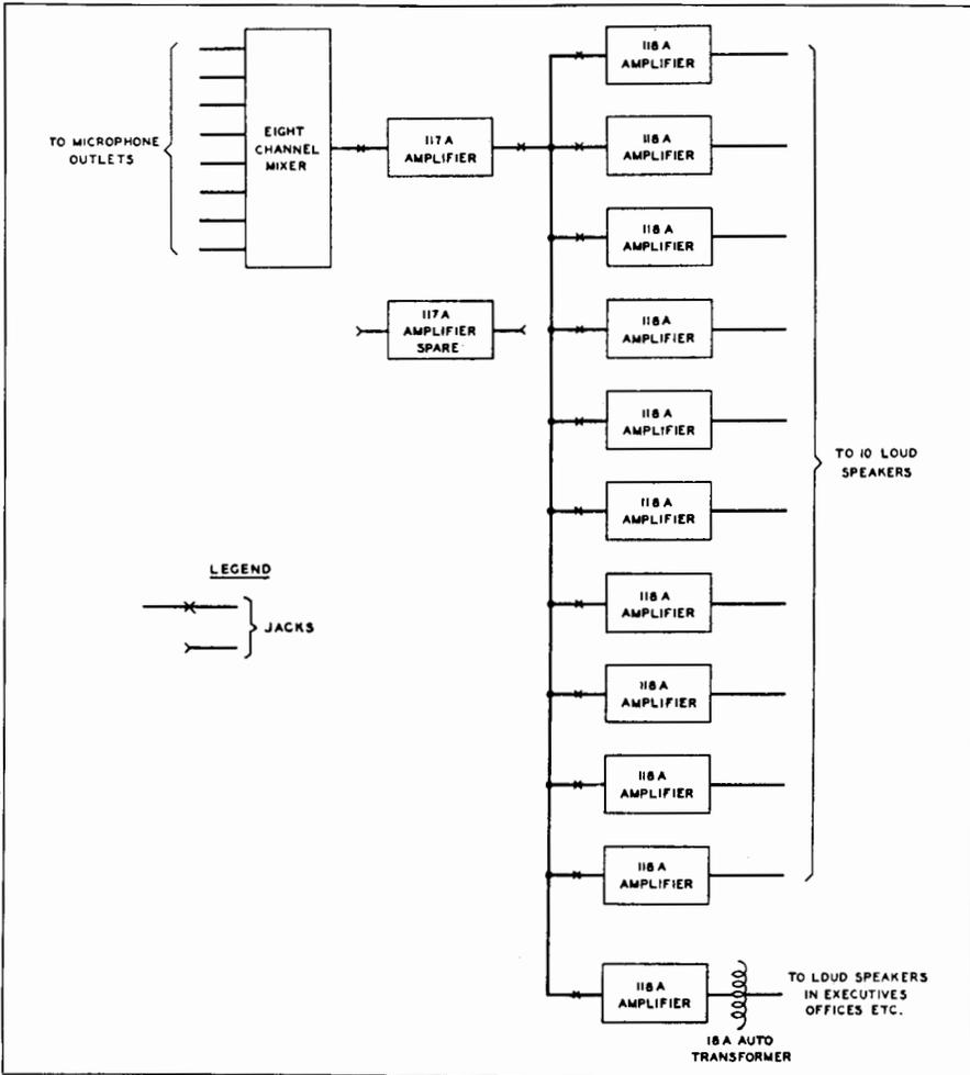
Fig. 22-7. Sound system for auditoriums requiring high levels.
