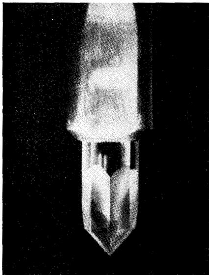
Fig. 7-23. Detail photo of the ANM V-groove stylus. (Courtesy, F. L. Capps)
