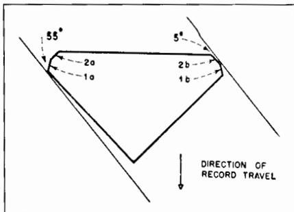
Fig. 7-14. Cross-section of same Anti-Noise Modulation Stylus in a groove whose slope is  $40^\circ$ . Leading facet 2b functions at an angle of  $5^\circ$  on the side where groove slope diminishes the burnishing angle. Facet 1a burnishes the opposite wall at  $55^\circ$ . (Courtesy, F. L. Capps)
