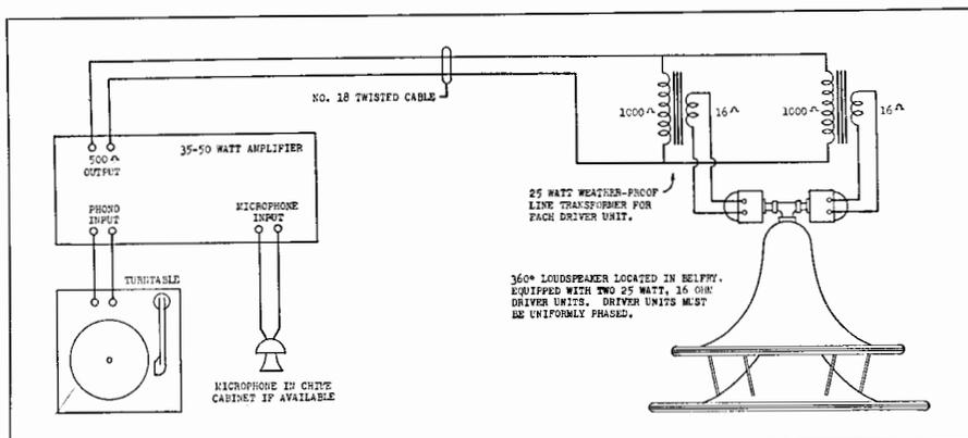
Fig. 22-14. A typical church steeple installation. (Courtesy University)
