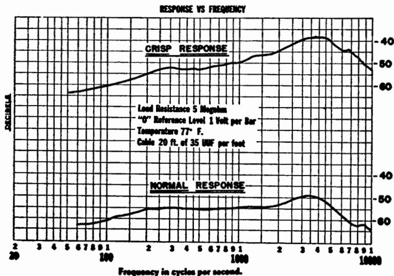
Fig. 14-20. Frequency response curves of the Astatic DR-10.
