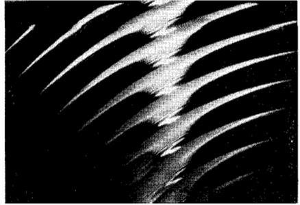
Fig. 28-9A. Clarkstan 102M microgroove audio sweep frequency record.
