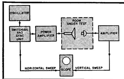
Fig. 23-6. Setup for performing transient acoustic measurements.
