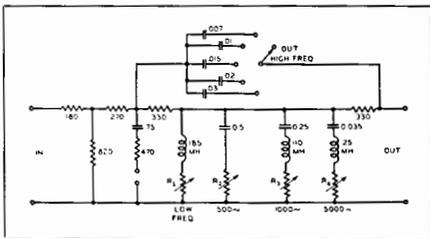
Fig. 5-29. Circuit diagram showing the final filter design.
