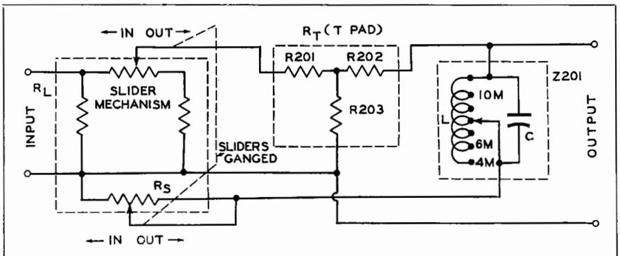
Fig. 18-3C. Simplified diagram of the Presto automatic equalizer.
