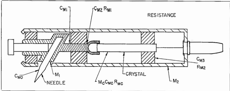
Fig. 9-26. Construction of the Bimorph type phono cartridge.
