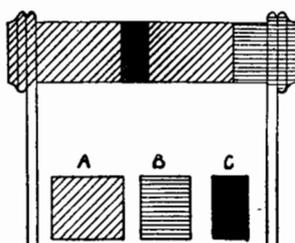
To identify a color coded resistor, locate the first two digits of the resistance value from Column A and B (Right). Find the number of zeros following the first two digits from Column C.
