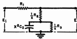
$$\text{LOSS} = 10 \text{ LOG } \left[ 1 + \frac{K^2 - 1}{1 + (f/f)^2} \right] + 10 \text{ LOG } K_L$$
