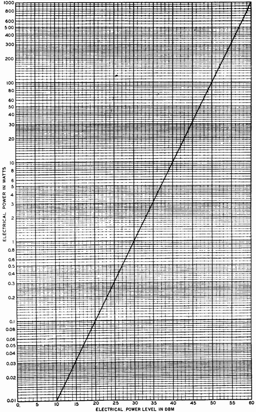
Fig. 22-4. Electrical power vs. electrical power level.
