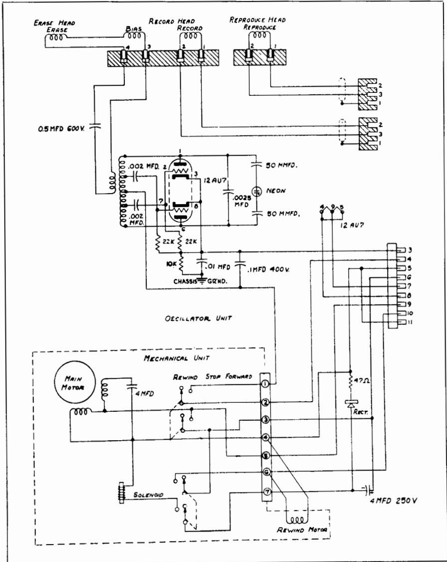
Fig. 12-36. Schematic of the Magnecoder PT63-A Oscillator Unit.
