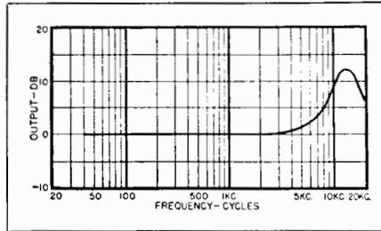
Fig. 3-15. Response of recording equalizer.
