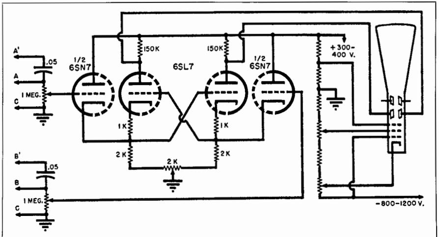
Fig. 19-17. Drive coupled push-pull amplifier suitable for push-pull or single ended input or for viewing point between the plates above ground.
