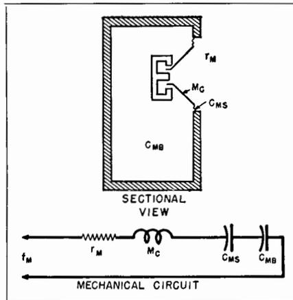
Fig. 15-30. Sectional view and mechanical circuit of a direct radiator loudspeaker mechanism mounted in a completely enclosed cabinet. In the mechanical circuit  $F_m$  = driving force,  $r_m$  = mechanical resistance of air load and suspension system,  $M_c$  = mass of the cone, voice coil, and air load.  $C_{MS}$  = compliance of the suspension system, and  $C_{MB}$  = compliance due to the cabinet volume.
