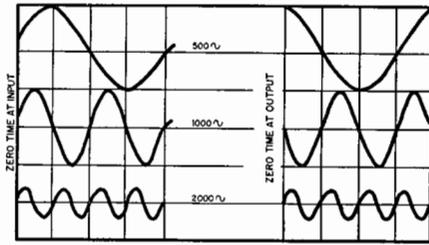
Fig. 28-14. Input and output phase relationships with theoretical linear phase shift of  $0.18^\circ$  per cycle. Note that time delay is constant at all frequencies—hence resultant waveform will not be changed.
