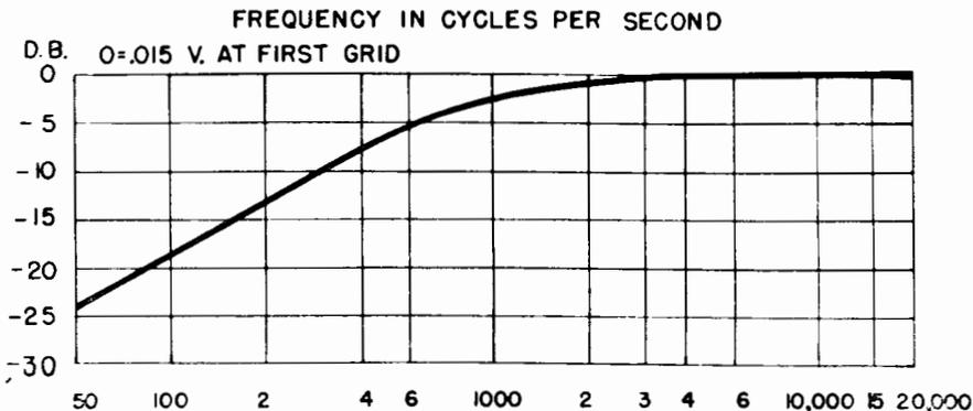
Fig. 12-37. Frequency response curve of the PT63-A.
