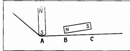
Fig. 11-24. Magnets arranged to provide three pole erasure.
