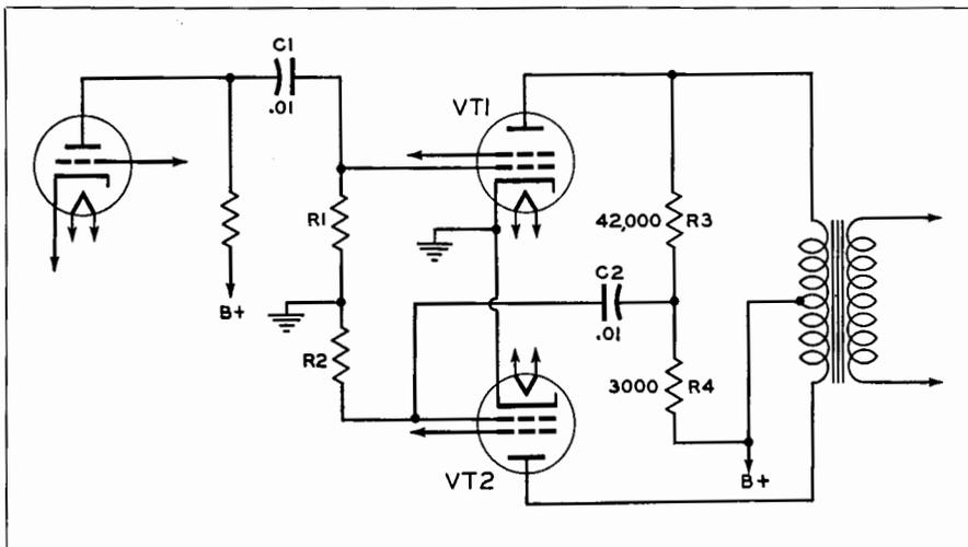
Fig. 19-7. Phase inversion takes place in the output stage. This system has the advantage of not requiring an inverter tube or additional transformers.
