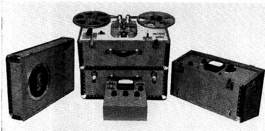
Fig. 13-12. Rangertone R-5PM synchronous tape recorder. (Courtesy Rangertone)
