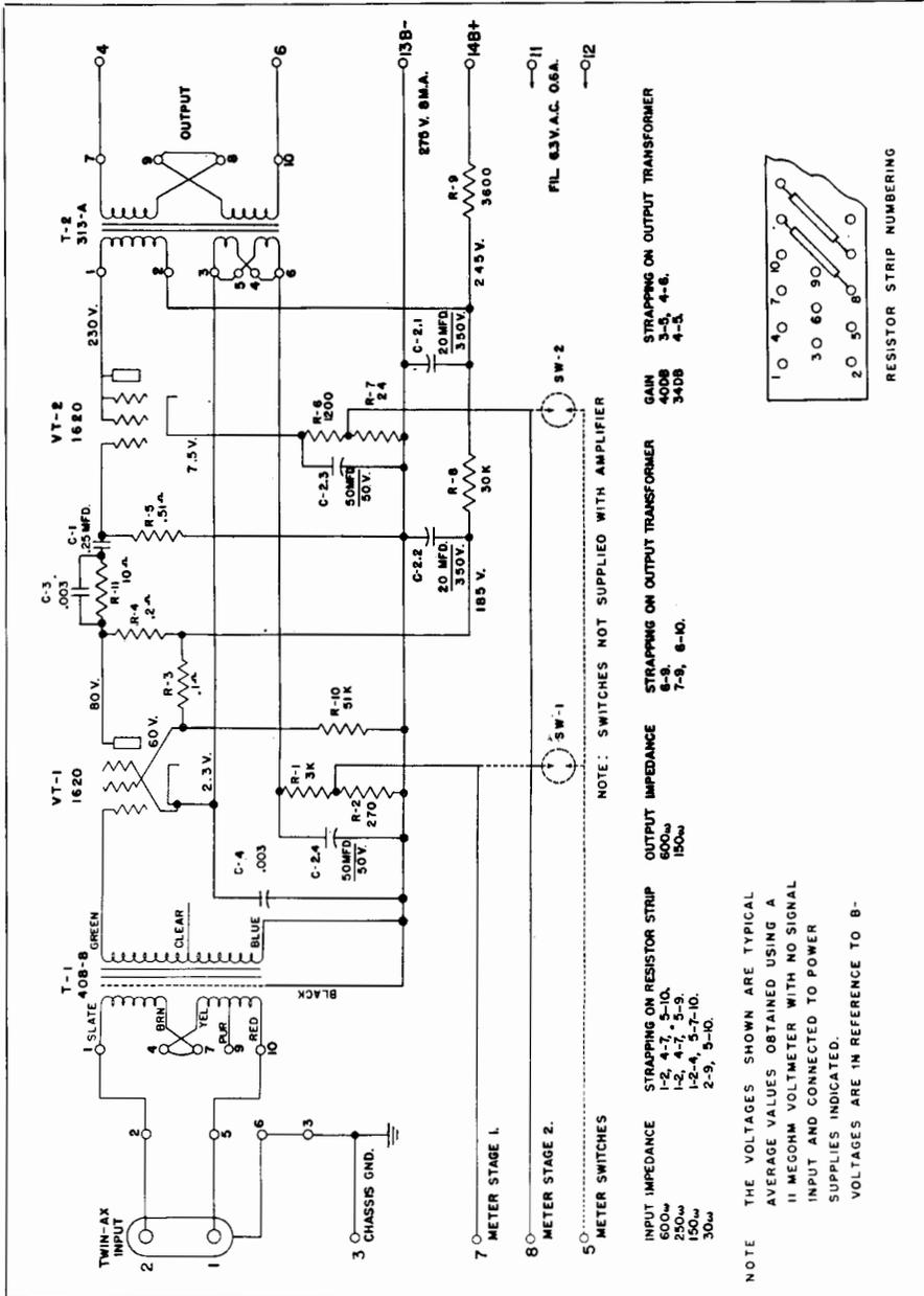
Fig. 25-12. Schematic of the Langevin 116-B booster amplifier.
