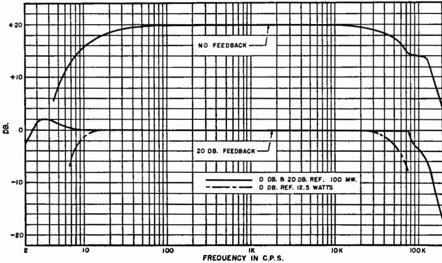
Fig. 21-6. Frequency response characteristics of the amplifier.
