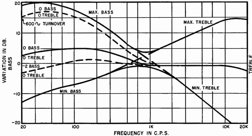
Fig. 26-7. Typical curves of the AE-2 preamp-equalizer.
