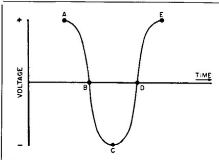
Fig. 11-2B. Waveform (output voltage) on recording head when wire is magnetized as in Fig. 11-2A. Peak voltage occurs when coil is at points  $A, C,$  and  $E.$  At  $B$  and  $D$  where there is no flux change, voltage is zero.
