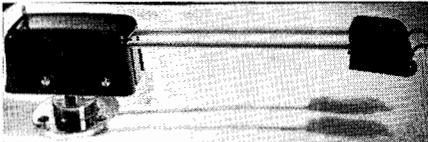
Fig. 10-11. The Goodell Duplex reproducer arm.
