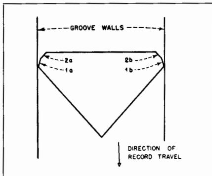
Fig. 7-13B. Cross-section of stylus shown in Fig. 7-13A in an unmodulated groove. The trailing facets 1a and 1b form burnishing angles of  $15^\circ$  with adjacent groove walls. (Courtesy, F. L. Capps)
