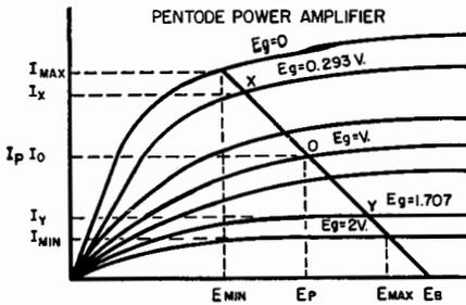
$$\text{POWER OUTPUT, WATTS} = \frac{[I_{MAX} - I_{MIN} + 1.41(I_X - I_Y)]^2 R_P}{32}$$
