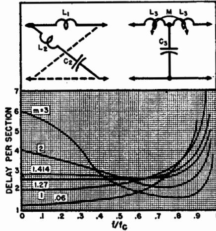
$$R_0 = \text{load resistance} = \sqrt{L_0/C_0}$$
