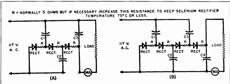
Fig. 19-29. (A) Voltage tripler circuit using three 200 ma. selenium rectifiers. With 40 mfd for  $C_1$ ,  $C_2$ , and  $C_3$ , a dc output of 325 volts can be obtained with a load of 200 ma. (B) Voltage quadrupler circuit using four 200 ma. selenium rectifiers. With 40 mfd for  $C_1$ ,  $C_2$ ,  $C_3$ , and  $C_4$ , a dc output of 425 volts can be obtained at 200 ma.
